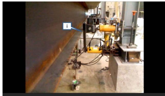
B) Image of video prior to actuator deflection of beam
